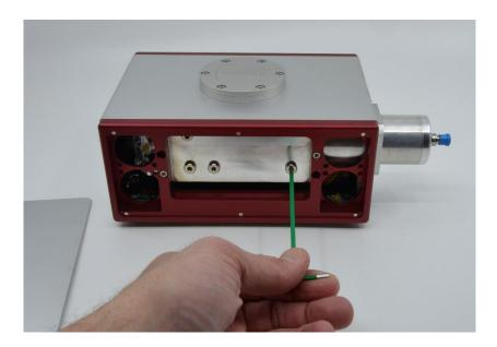
Finally, replace at least one of the screws by the push-in fitting, and connect the purge tube. Use a low volumetric flow, in the order of 0.5L/min or less.
